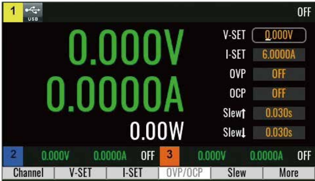
Single-Channel Meter Interface and Quick Setup Interface
